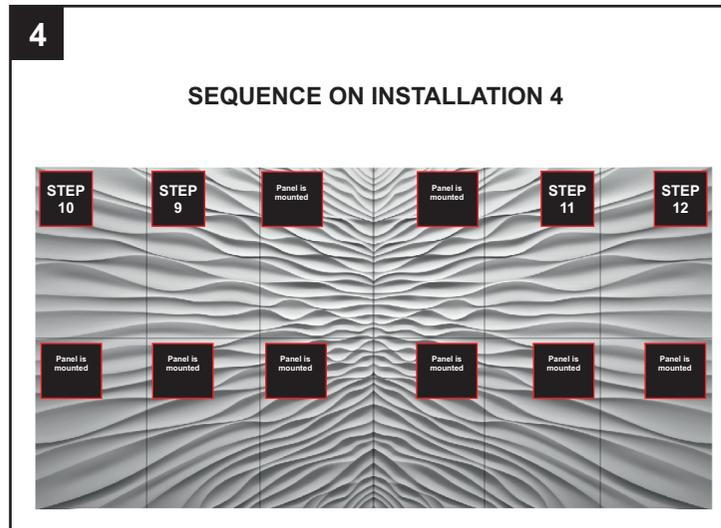
The final step of installation is to mount panels 9, 10 and 11, 12. After mounting, next day you can fill joints, cleaning, painting and that's all :-)
