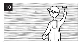
Before painting, panels should be prime by WeldPrimer by using a velor
