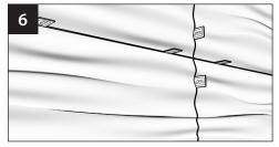
Gluing individual panels (keep the distance between the panels from 1.5 to 3 mm). Another layers of panels mounted after making sure that the previous layer is permanently mounted. For high-quality installation, use the original cardboards.
