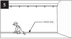
Starter strip is necessary just if panels will be install above the level of floor. The starting strip should be made of solid, non bending material.
