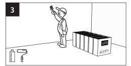
Preparing the wall. Prim the wall with WeldPrimer, and if the surface is slippery use Joni Grip.
